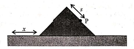
At the right end P of the chain, a mass m is attached. The system is subjected to the gravity force and we ignore friction. At time t = 0 it is at rest with a length s(0) = 1/2 of chain lying from the right side of the block. Write down the Lagrangian of the system.
